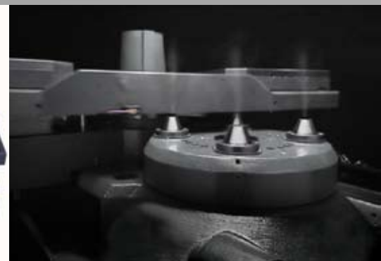
■ Discharging air jet pallet indexing system
