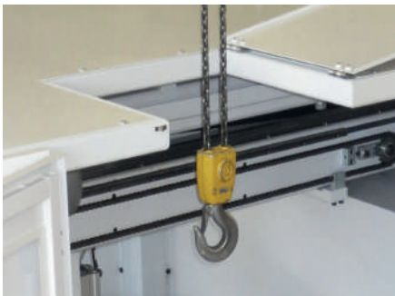
Top loading door for crane operation.
