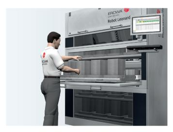
Pallets are moved into the robot via the integrated loading station. Leonardo automatically places the prepared pallets into an available magazine position.
