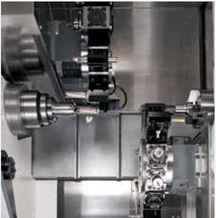
Upper-L/Lower-R Boring operation
