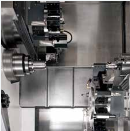
Upper-L/Lower-R Turning operation
